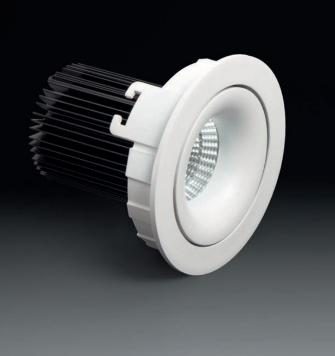
Biss is an adjustable recessed light characterized by a perfect and unobtrusive design. It is made from die-cast aluminium and equipped with a Chip On Board technology high efficiency LED light source and a remote driver. Its degree of protection against the penetration of dust, solid objects and liquids is IP23.
