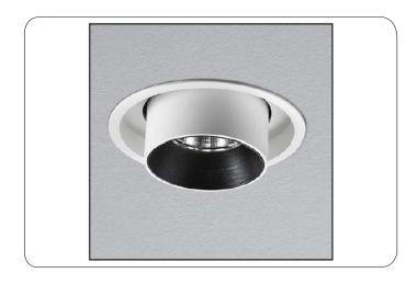
Recessed fixture which can be angled on two 360° and 90° axes and pulled out, complete with a high efficiency 10W LED source with a luminous flux of 800 lumen. Made of epoxy-polyester powder coated finish die-cast aluminium stabilized with UV rays. The fixture is supplied with a remote driver and it is available version DALI dimmable switch-dim. The degree of protection against the penetration of dust, solid object and liquids is IP23. Remote driver included.
