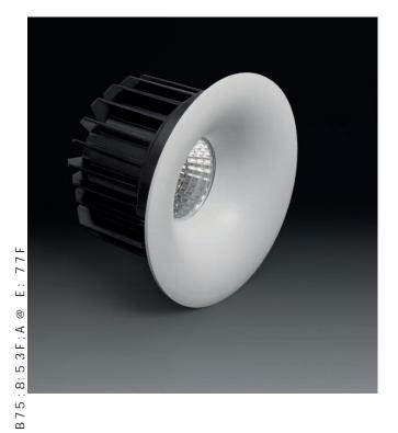
A curvy shape identifies Edo, a recessed light made from die-cast aluminium and equipped with a Chip On Board technology high efficiency LED light source and a remote driver. It is available in two sizes. Its degree of protection against the penetration of dust, solid objects and liquids is IP44. 40°
