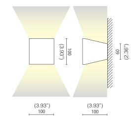
Characterized by the symmetrical cuts, Mia is a dou-ble emission wall lamp made from epoxy polyester powder coated aluminium and it is equipped with Chip On Board technology high efficiency LED light sources and driver. Its degree of protection against the penetration of dust, solid objects and liquids is IP20.
