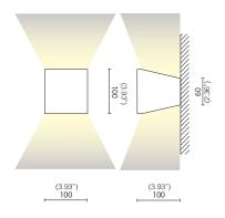
Characterized by the symmetrical cuts, Mia is a dou-ble emission wall lamp made from epoxy polyester powder coated aluminium and it is equipped with Chip On Board technology high efficiency LED light sources and driver. Its degree of protection against the penetration of dust, solid objects and liquids is IP20.
